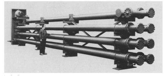
Continuous cooling crystallizers for fractional crystallizations and purifications. Typical duties include separation of aromatic isomers, fatty acid separations, edible fat fractionations, and purification of many organic intermediates. Construction in stainless and carbon steel, nickel alloys, hastelloy, etc. Construction to ASME, TUV, Stoomwezen, and other international codes. Test units available to rent to prove out new processes.
